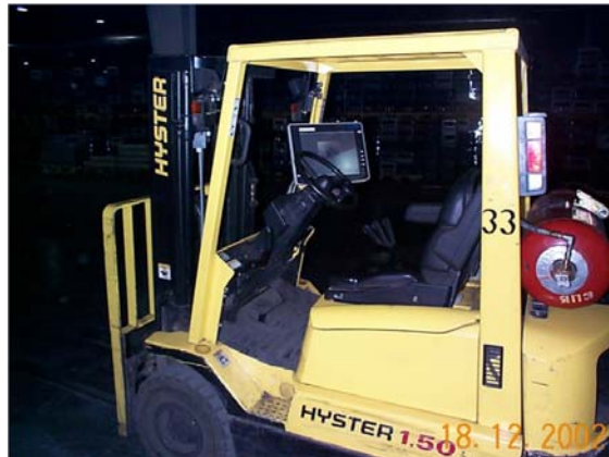
Figure 6.2: The mobile PC mounted on an forklift
